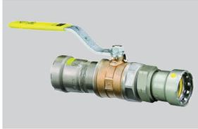
The MegaPressG ball valve comes equipped with a full port silicon bronze body, a 316 stainless steel ball, and zinc-nickel-coated steel press ends. The ball valve is PxGJ and features an HNBR sealing
