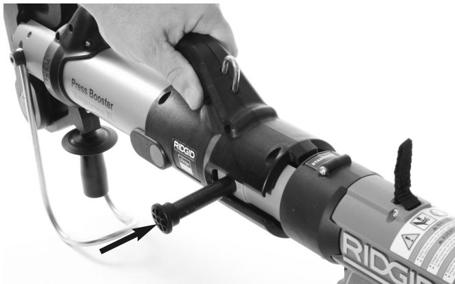
Figure 2 – Installing Press Booster on Press Tool
