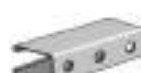
AS 150H Channel with Holes Size: 1 1/8" x 2 7/16" x 12 GA. 9/16" Holes on 1 7/8" Centers.
