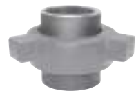
Fig. 3L31A Tri-Lug High Speed Union 3,000 psi cwp - 4,500 psi test Size Range: 1" - 2"
