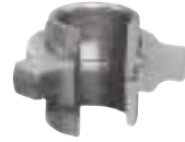
Fig. 211 Threaded Ends Insulating Union 2,000 psi cwp - 3,000 psi test Sizes: 1" & 2"
