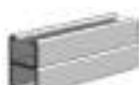
AS 200EH BTB Welded Channel Size: 1 1/8" x 3 1/4" x 12 GA. Two Pcs. AS 200EH Welded Back-to-Back. 9/16" x 1 1/8" Elongated Holes on 2" Centers.
