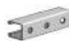
AS 200H Channel with Holes Size: 1 1/8" x 1 7/8" x 12 GA. 9/16" Holes on 1 7/8" Centers.
