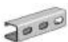
AS 300EH Channel with Elongated Holes Size: 1 1/8" x 1 3/8" x 12 GA. 9/16" x 1 1/8" Elongated Holes on 2" Centers.
