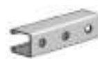
AS 210H Channel with Holes Size: 1 1/8" x 1 1/8" x 14 GA. 9/16" Holes on 1 7/8" Centers.
