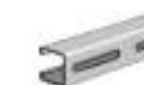
AS 200S Channel with Long Slots Size: 1 1/8" x 1 7/8" x 12 GA. 1 3/32" x 3" Slots on 4" Centers.
