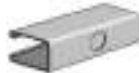
AS 150KO Channel with Knock Outs Size: 1 1/8" x 2 7/16" x 12 GA. 1 1/8" Knock Outs on 6" Centers.
