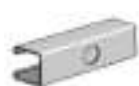
AS 300KO Channel with Knock Outs Size: 1 1/8" x 1 1/8" x 12 GA. 7/8" Knock Outs on 6" Centers.
