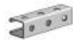
AS 200H3 Channel with Holes on all Three Sides Size: 1 1/8" x 1 7/8" x 12 GA. 9/16" Holes on all three sides are on 1 7/8" Centers.
