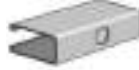
AS 100KO Channel with Knock Outs Size: 1 1/8" x 3 1/4" x 12 GA. 7/8" Knock Outs on 6" Centers.
