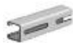
AS 210S Channel with Long Slots Size: 1 1/8" x 1 1/8" x 14 GA. 1 3/32" x 3" Slots on 4" Centers.
