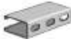
AS 100EH Channel with Elongated Holes Size: 1 1/8" x 3 1/4" x 12 GA. 9/16" x 1 1/8" Elongated Holes on 2" Centers.
