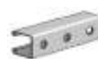
AS 300H Channel with Holes Size: 1 1/8" x 1 3/8" x 12 GA. 9/16" Holes on 1 7/8" Centers.
