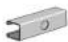
AS 210KO Channel with Knock Outs Size: 1 1/8" x 1 1/8" x 14 GA. 7/8" Knock Outs on 6" Centers.
