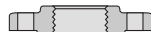
Fig. 1025 Cast Iron Companion Flange Size Range: 1¼" x 5¼" thru 8" x 15" NPS
