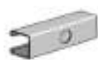
AS 200KO Channel with Knock Outs Size: 1 1/8" x 1 7/8" x 12 GA. 7/8" Knock Outs on 6" Centers.
