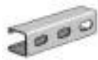
AS 210EH Channel with Elongated Holes Size: 1 1/8" x 1 1/8" x 14 GA. 9/16" x 1 1/8" Elongated Holes on 2" Centers.
