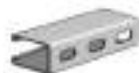
AS 150EH Channel with Elongated Holes Size: 1 1/8" x 2 7/16" x 12 GA. 9/16" x 1 1/8" Elongated Holes on 2" Centers.
